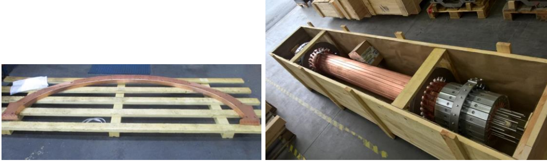
FIG.8. Toroidal field magnet: one of 24 return limbs, left, and the central post, right.
