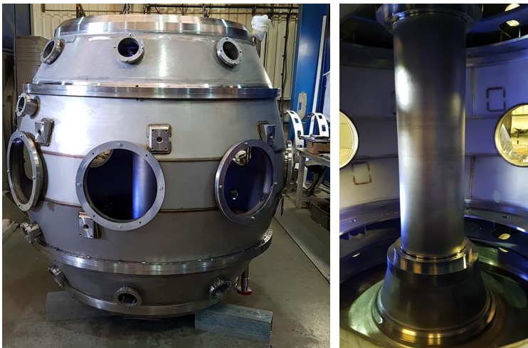
FIG.4. ST40 vacuum vessel. General view, left and view from inside, right. Divertor, internal diagnostics and graphite tiles are not installed.
