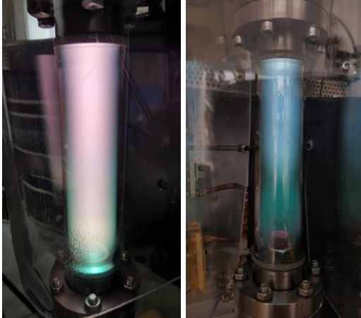
FIG.6. Left: RF glow discharge in He gas with the BN dish filled with crystalline boron at the bottom; right: Li evaporation experiments with RF discharge in He.
