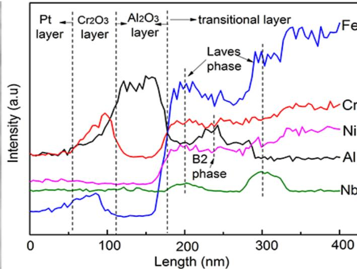
Thin Cr-oxide layer followed by Al-Oxide scale - < 50nm after 2000h
