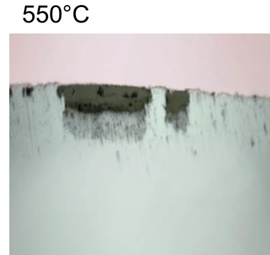
Up to 600°C and 1 corrosion attack and no visible oxidation. Fe<sub>12</sub>Cr<sub>7</sub>Al
