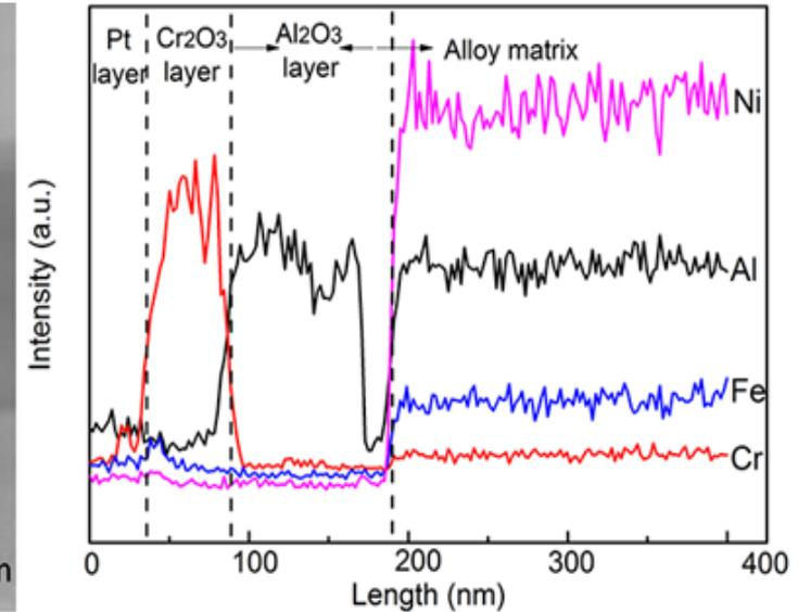
All specimens besides the Cu containing show the formation of a protective oxide scale mainly AlCr rich.
