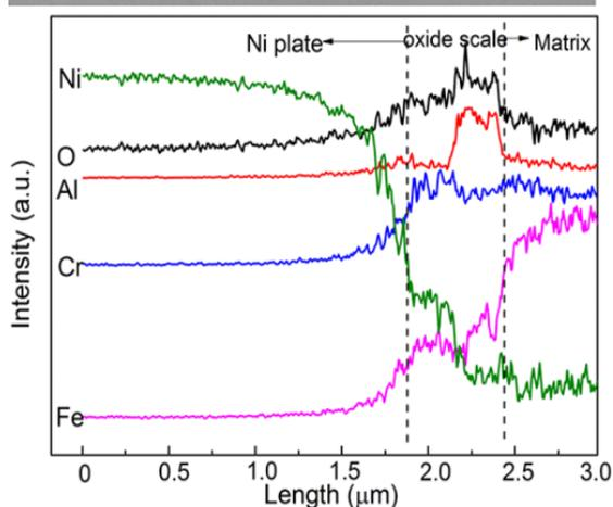
All specimens besides the Cu containing show the formation of a protective oxide scale mainly AlCr rich.
