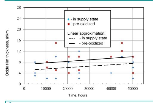
Bench corrosion testing of fuel rod models in the flow of coolant lead-bismuth was carried out on two identical loops SM-1 and CU-2M in the SSC RF-IPPE at the design values of the dissolved oxygen concentration and maximum circulation velocity of the alloy
