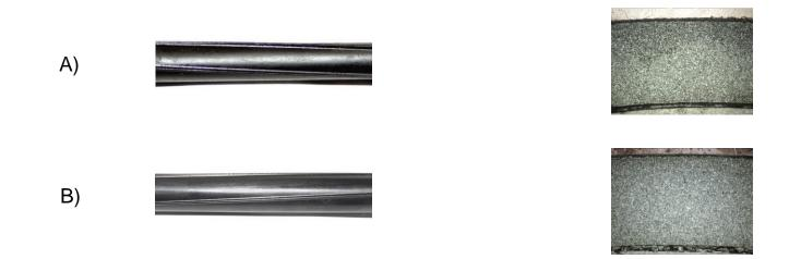
Appearance of samples and microstructure of material after tests in Pb-Bi:
