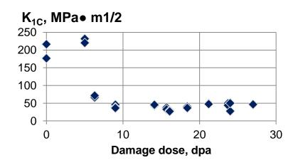
Under such criteria, the damaging dose to the materials of reactor internals should be limited to the value of  $6\div 8$  dpa. To meet the accepted criterion, the design of the reactor was modified with changes in both the design of the reactor and the use of materials for its elements.
