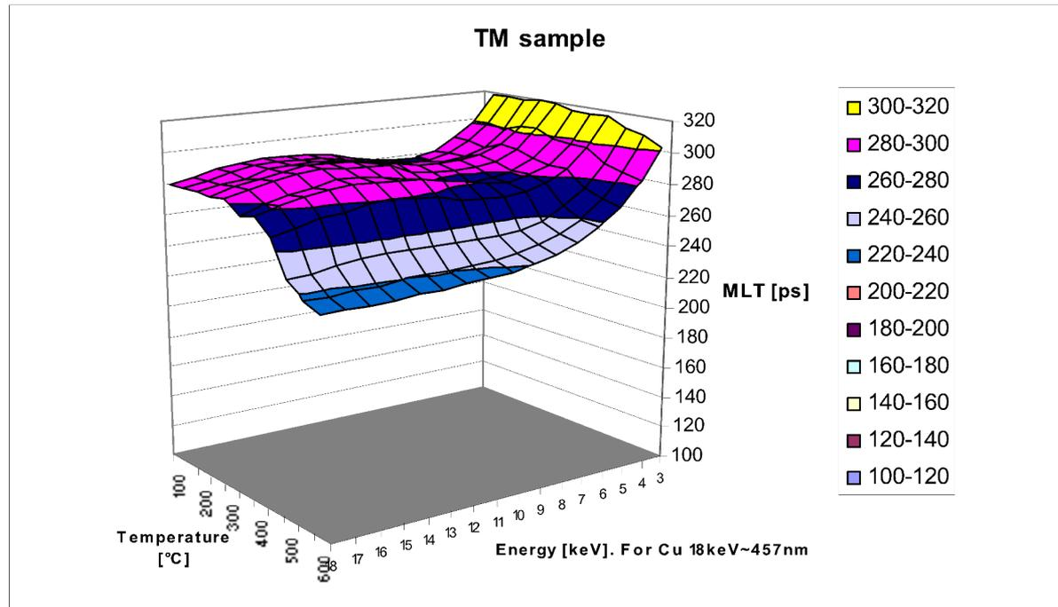
Annealing behaviour of irradiated CuAl<sub>25</sub>-sample (TM)
