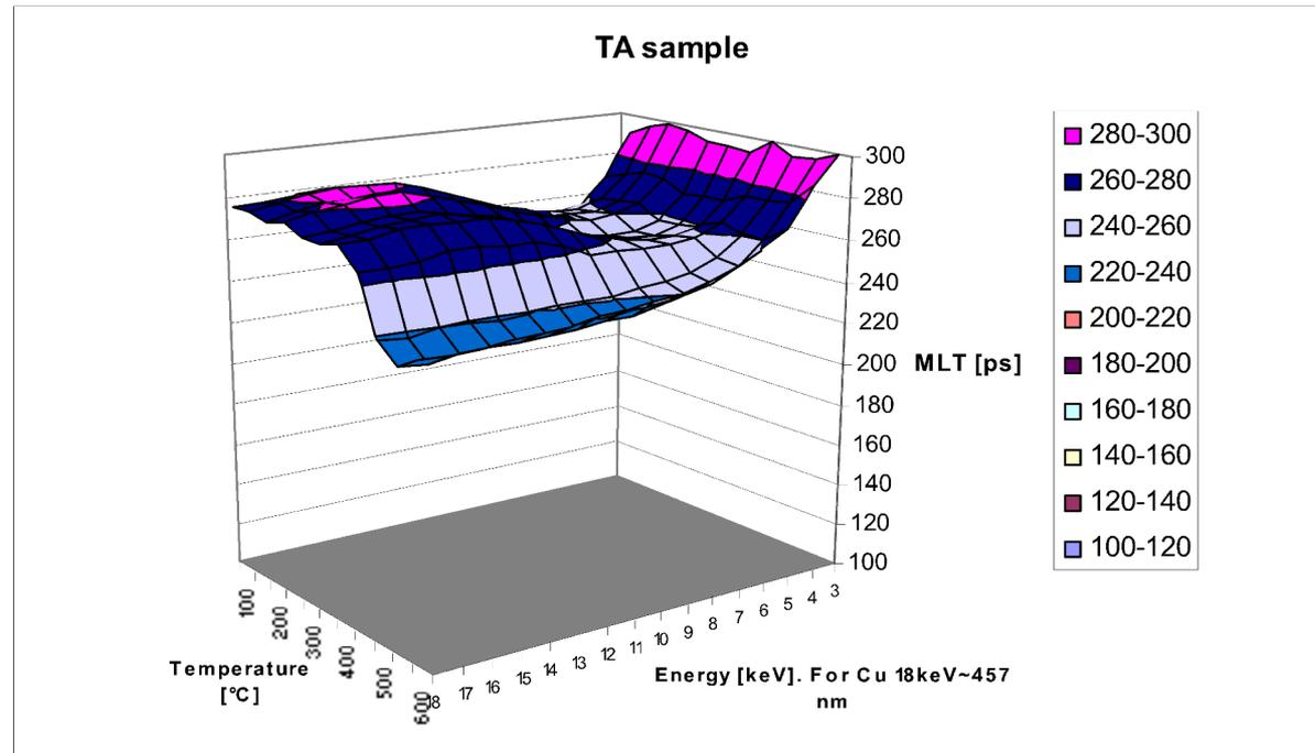
Annealing behaviour of irradiated CuAl<sub>25</sub>-sample (TA)
