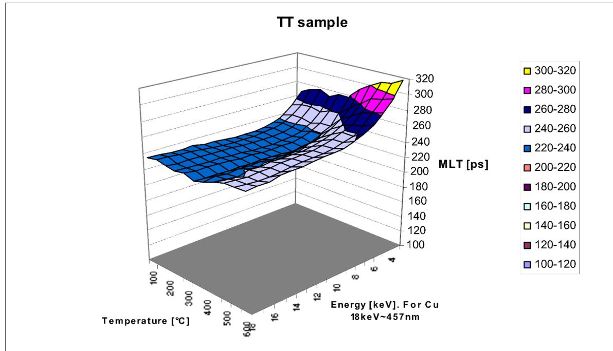
Annealing behaviour of irradiated CuAl<sub>25</sub>-sample (TT)
