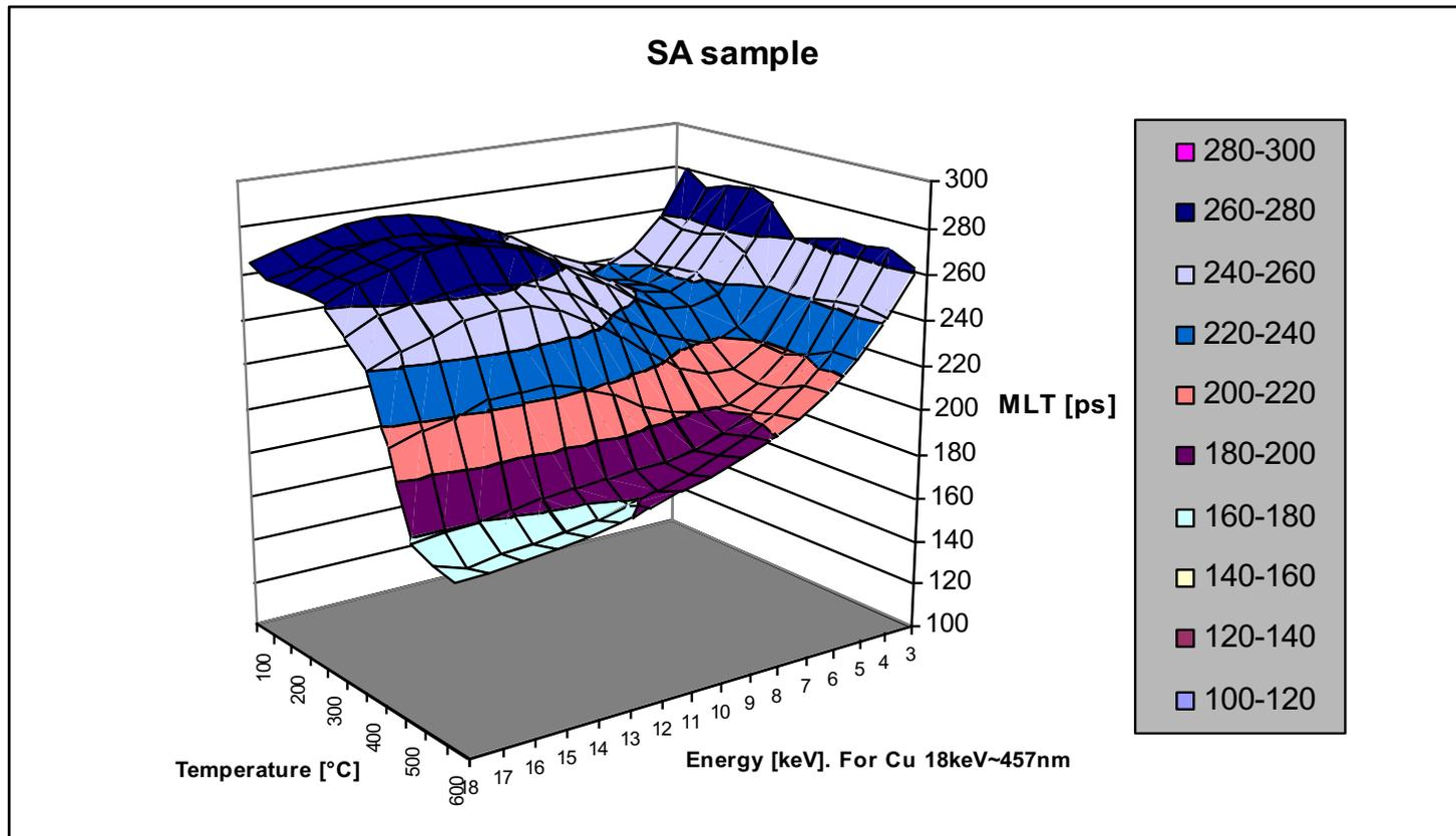
Annealing behaviour of irradiated CuCrZr-sample (SA)
