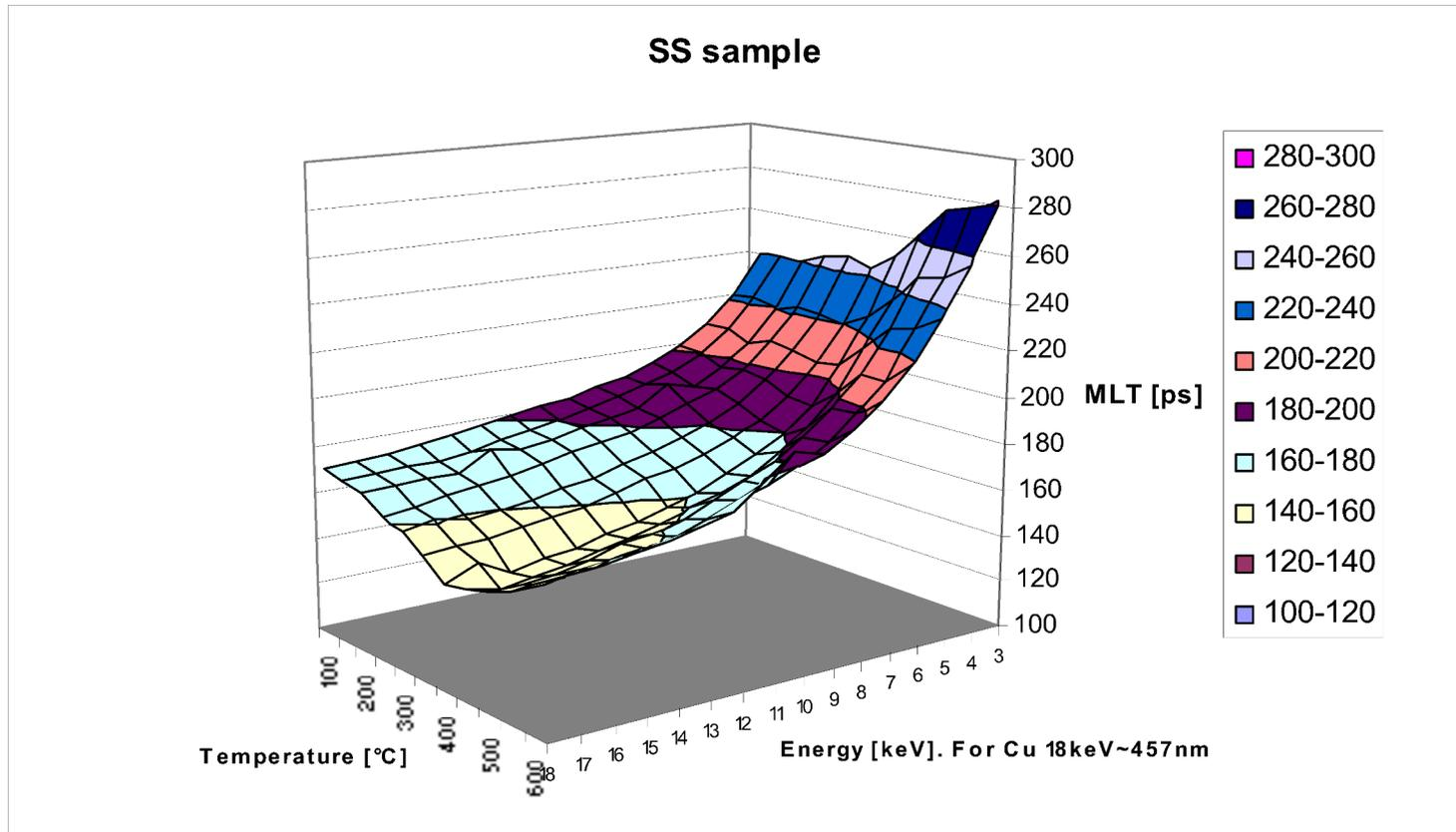
Annealing behaviour of not-irradiated CuCrZr-sample (SS)
