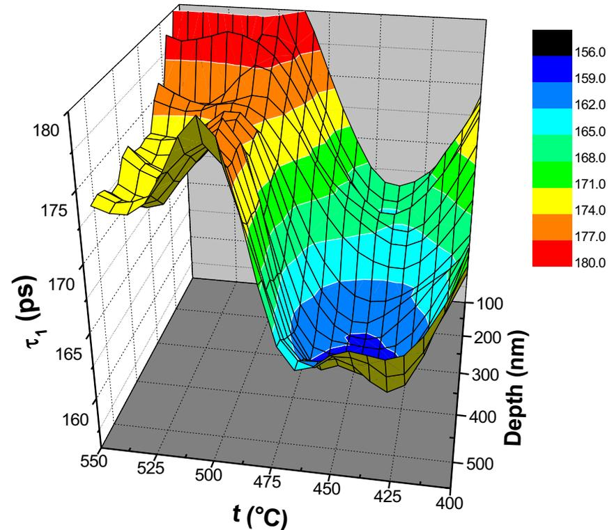
The 3D presentation of PLEPS results ( $\tau_1$ ) of irradiated ( $1.25 \times 10^{24} \text{m}^{-2}$ ) and annealed Sv-10KhMFT steel (WWER-440 weld).
