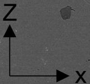
SEM confirms the PLEPS results of large voids in the depth  $>500\text{nm}$  which correspond to the implantation profile maxima .
