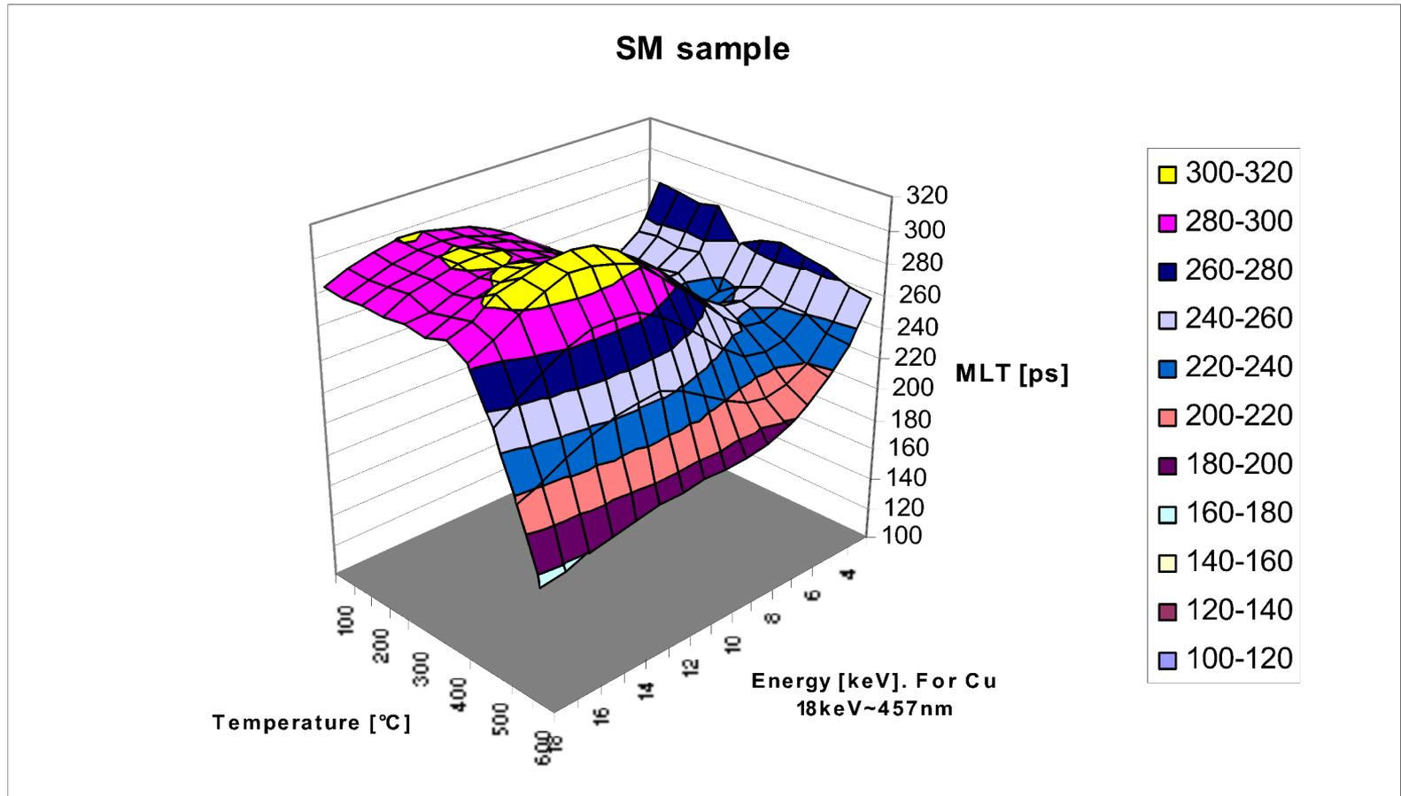
Annealing behaviour of irradiated CuCrZr-sample (SM)
