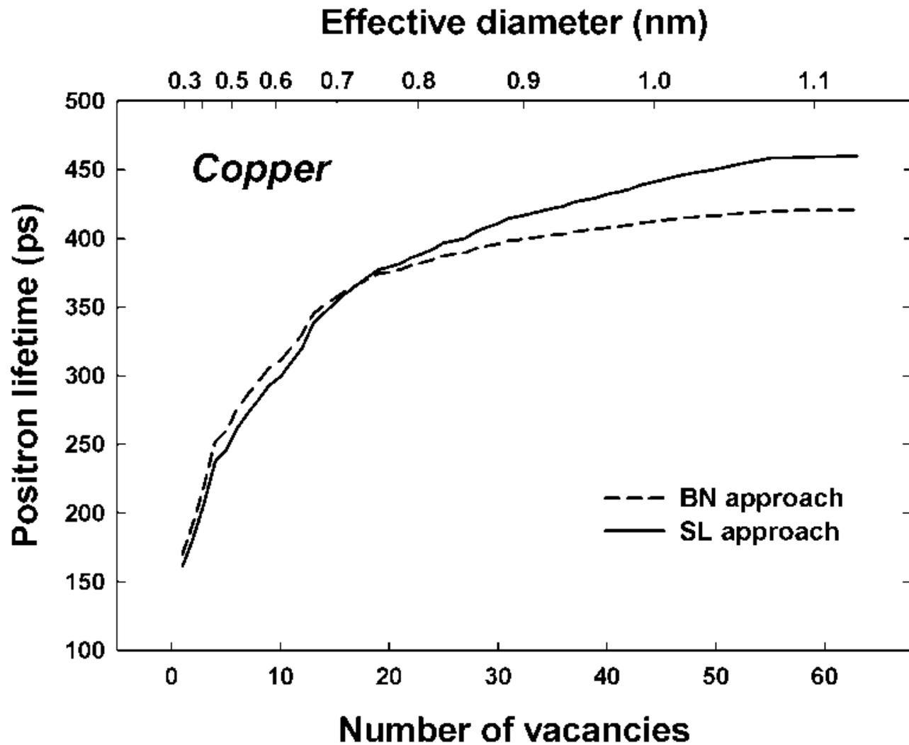
The calculated dependence of the positron lifetime on the size of the vacancy cluster in Cu.
