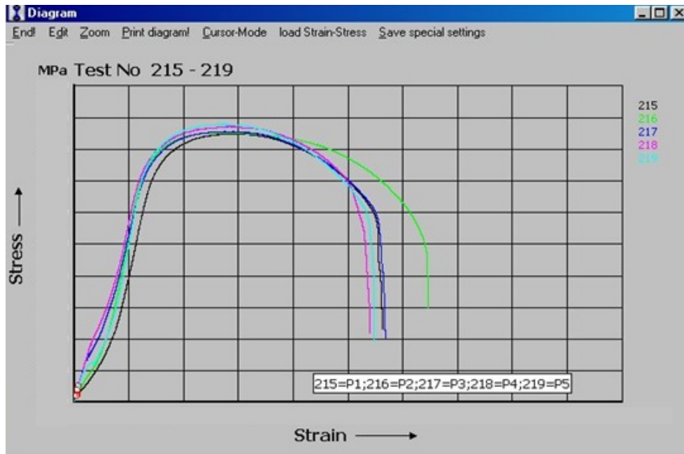
The stress-strain tensile curves for coated T91 specimens
