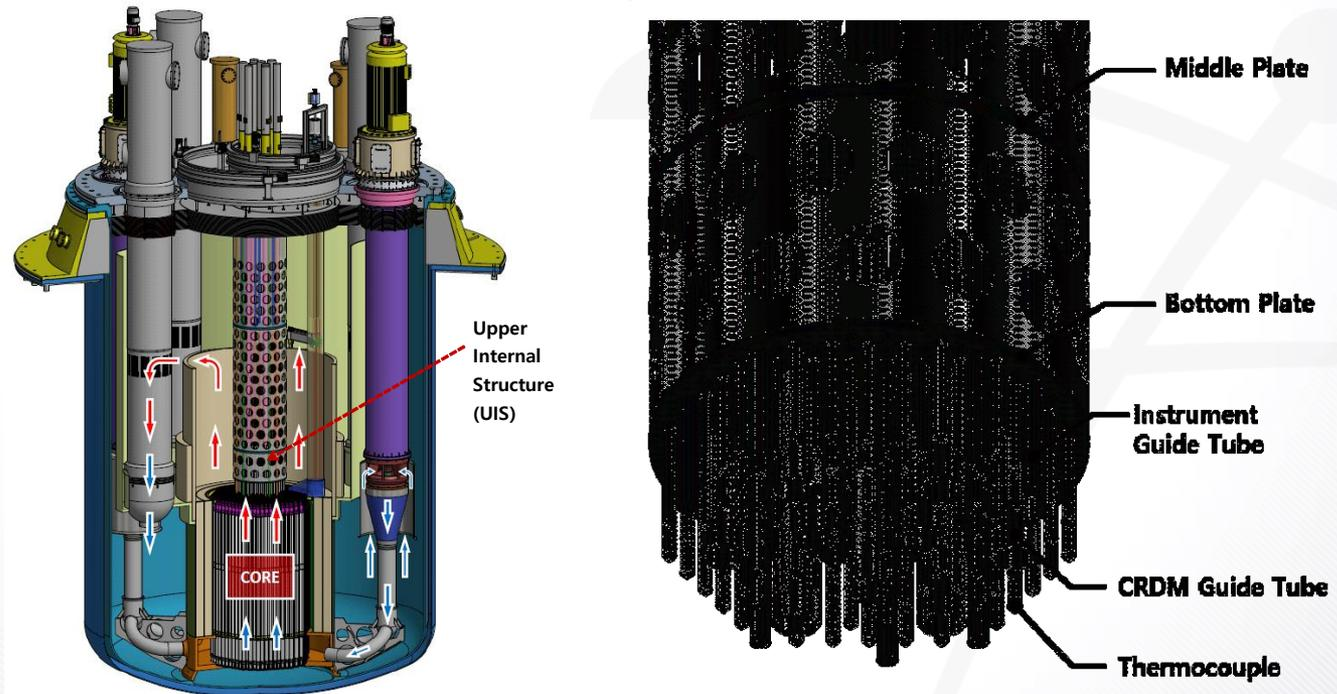
Schematic diagram of the reactor core and close-up view of the upper internal structure
