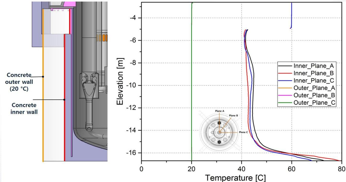
Vertical temperature distribution of inner & outer concrete in the RVCS
