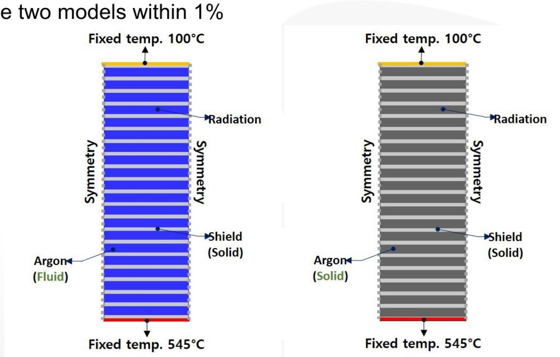
Simplified modelling of the upper shield structure (Left: Original, Right: Argon region as solid)
