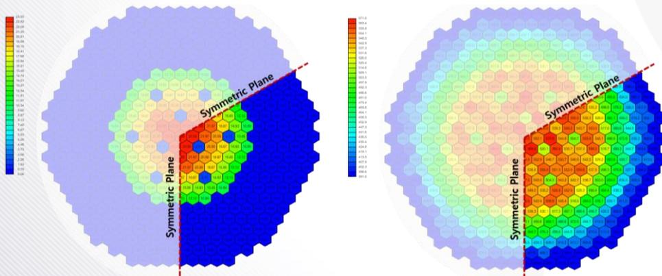
Core exit flow conditions of computation region (Left: Flow rates, Right: Temperatures)
