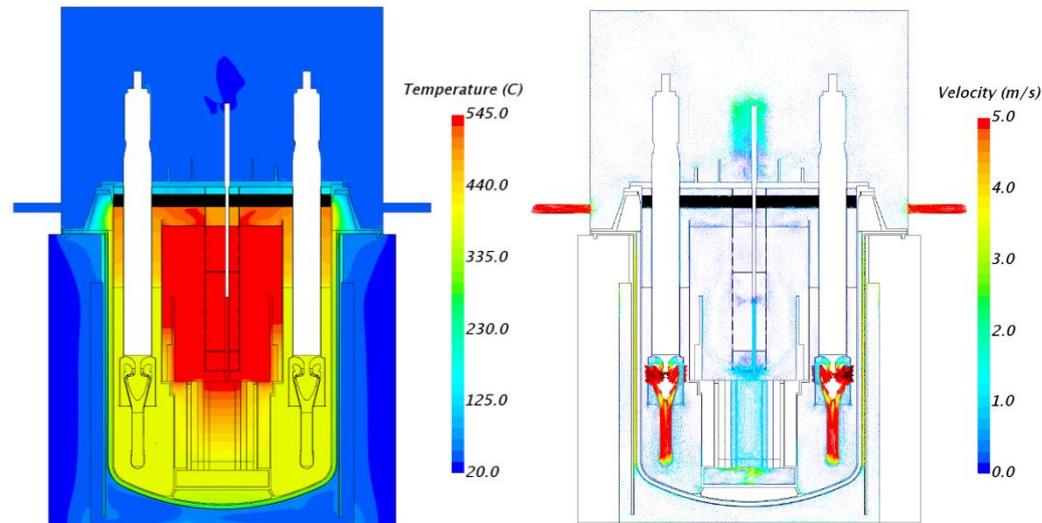
Temperature distribution (left) and velocity distribution (right)
