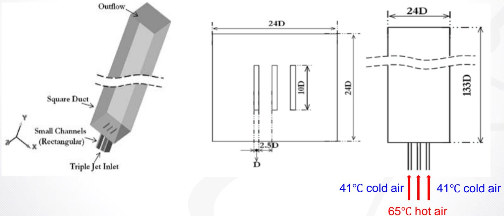
Schematic diagram of triple jet geometry
