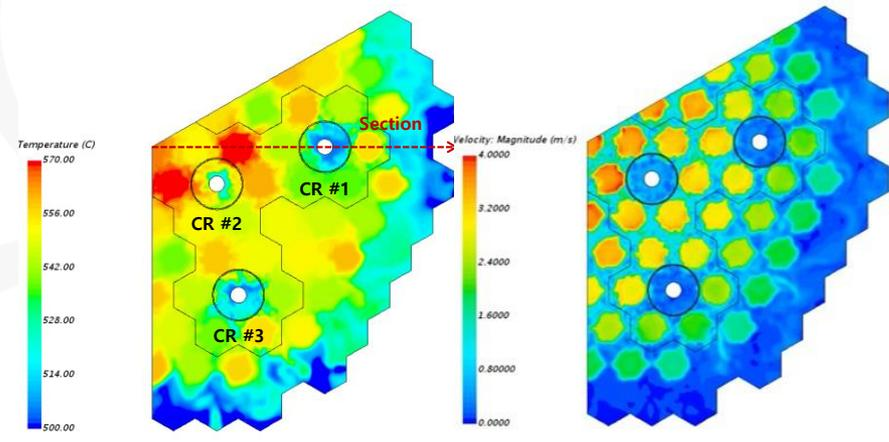
Temperature and velocity distribution at the horizontal section (50 mm off from the core exit)
