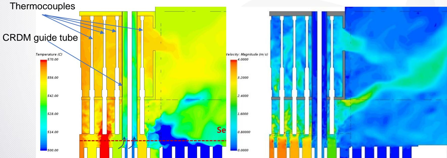
Temperature and velocity distribution at the vertical section through CR #1
