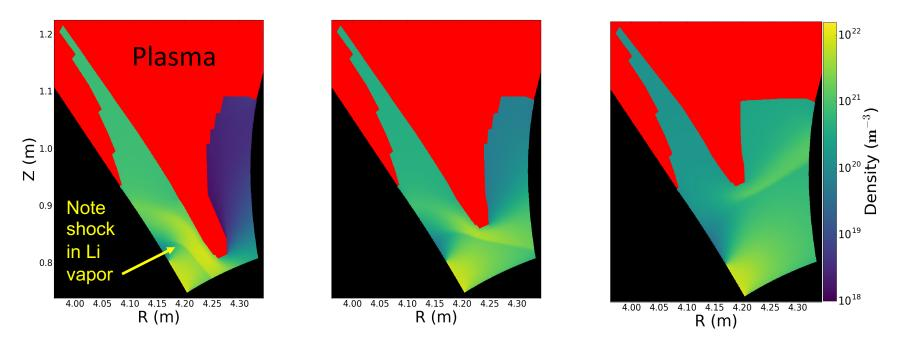
Factor of 6 reduction in lithium ionization as plasma retreats from vapor region  $\Rightarrow$  stable detachment front
