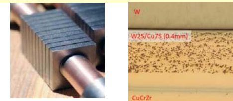
Thin graded interlayer ( W/Cu )
