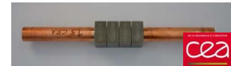
FGM- Graded interlayer (W/Cu: 20μm, 400μm)
