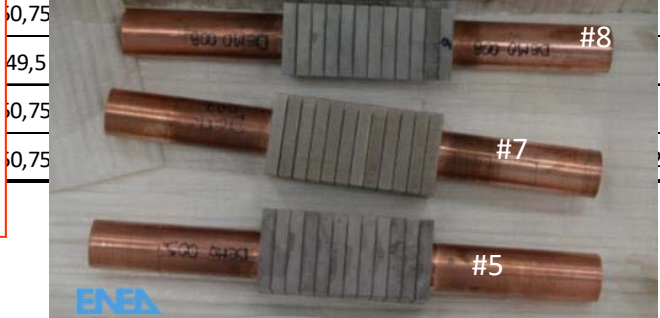
W+CuCrZr pipe: ITER-like 1mm Cu-interlayer
