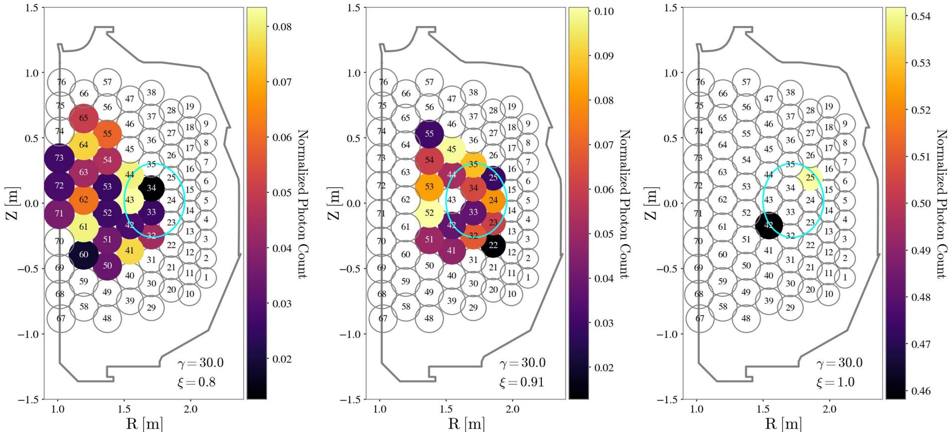
It will be harder to measure centrally peaked distributions at pitch close to one due to fewer sensitive chords and smaller orbits
