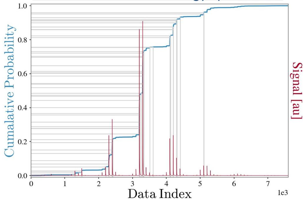
The GRI uses pulse height counting over a fixed time period to generate a distribution of photon energies
