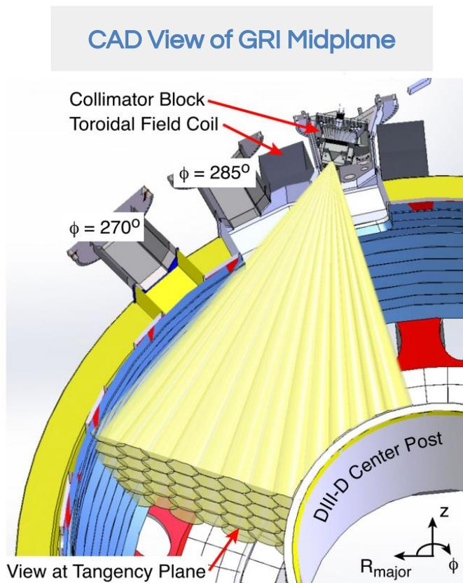
The Gamma Ray Imager is a pinhole camera with multiple pulse height counting detectors that are used to build up a histogram of photon energies over an integration time  $\sim 100\text{ms}$
