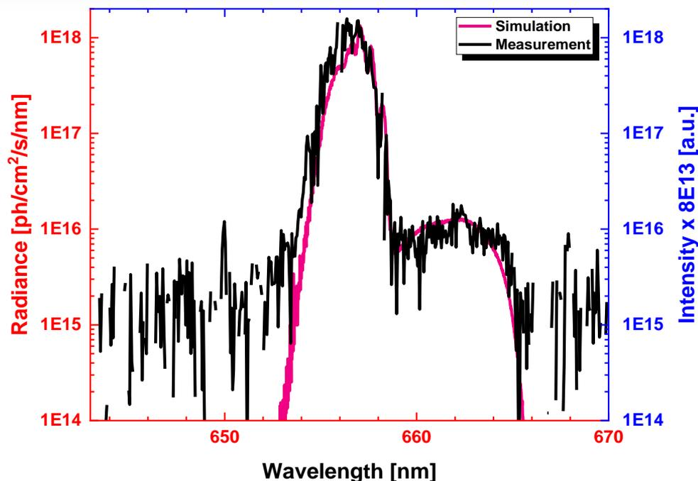
In this experiment, H/D ratio was 0.23/0.77 that was measured by H $\alpha$  and D $\alpha$  intensity.
