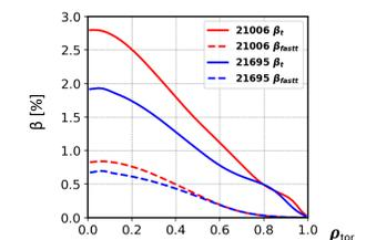
Even 21006 has more NB power, its perpendicular components could lead an ineffective NBCD.
