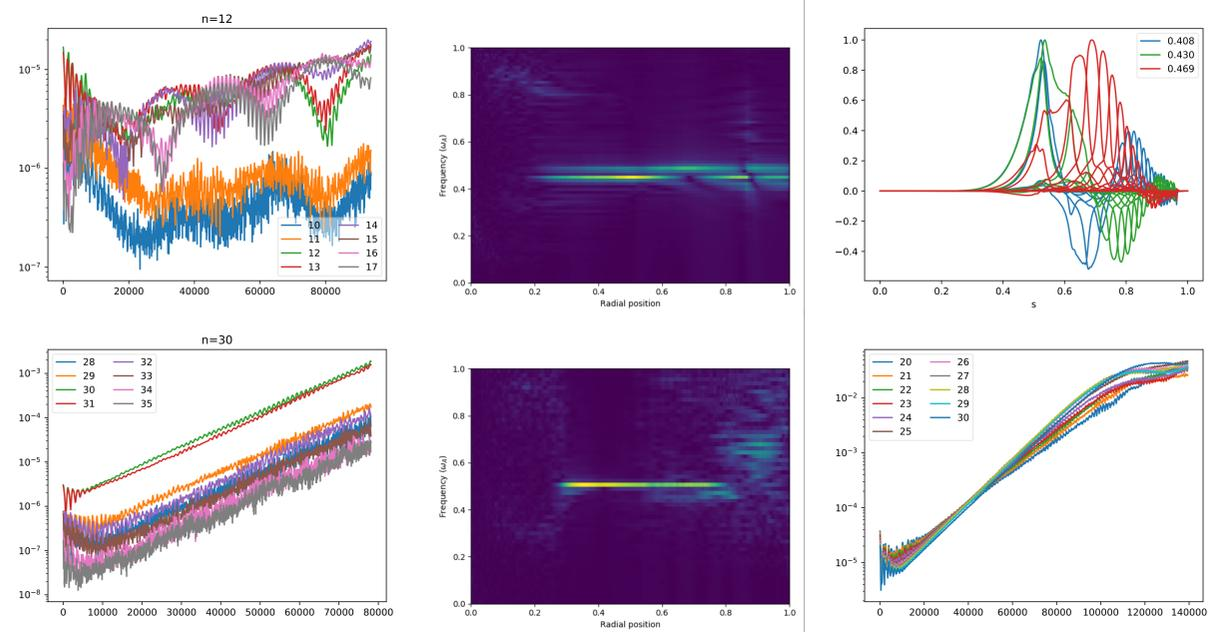
Fig. 2 (Upper):  $n = 12$ : Evolution of the harmonics of the electrostatic potential (left), spectrogram (middle). We compare these to eigenfunctions obtained from LIGKA (right).
