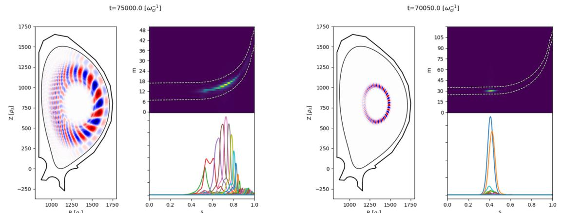
Fig. 1: Snapshots of the electrostatic potential for TAEs with  $n = 12$  (left) and  $n = 30$  (right).  $R / Z$  are in units of  $\rho_s$ .
