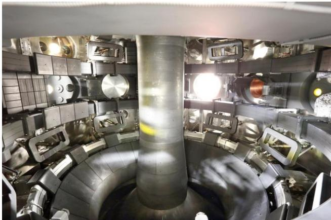
Figure 6: Photograph of the completed interior of MAST Upgrade prior to being pumped down.
