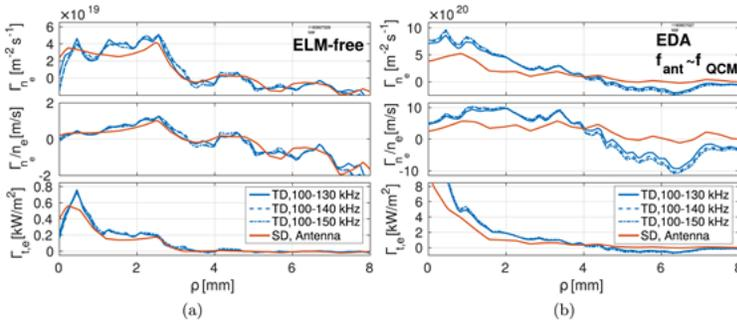
Fig. 5.4 Profiles of radial transport of particles ( $\Gamma_n$ ,  $\Gamma_n/n_e$ ) and energy ( $\Gamma_e$ ) driven by a QCM-like mode driven by the Shoelace antenna during ELM-free (left) and EDA phases (right) of ohmic H-mode plasmas. Mirror Langmuir probe data are analyzed using time domain analysis (TD) in three frequency bands and via a spectral domain (SD) analysis.  $\rho$  is the distance from the last closed flux surface at the outer mid plane.
