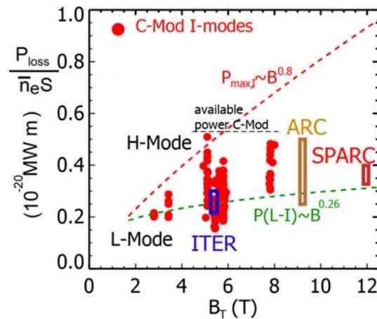
Fig. 3.2 I-mode operation in C-Mod in the space of power/area vs. toroidal field. Also shown are predictions for ITER, and two future concepts, SPARC and ARC.
