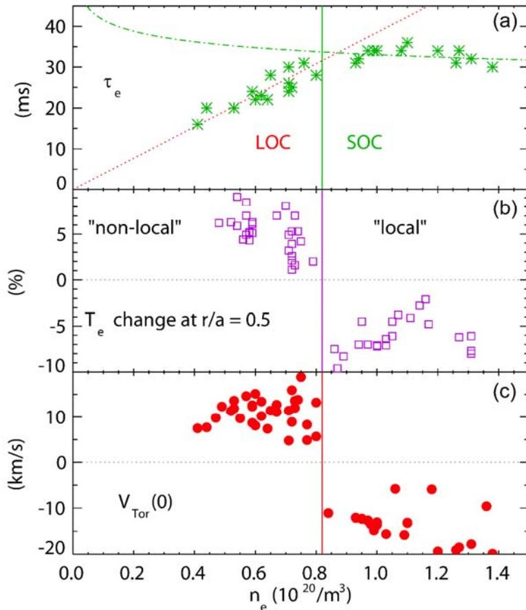
Fig. 2.2 Density dependence of plasma responses across the LOC/SOC boundary: a) scaling of  $t_e$ ; b)  $T_e$  response at  $r/a=0.5$  after edge impurity injection, showing the “non-local” ~5% temperature rise in the LOC regime; c) reversal of intrinsic core rotation across the boundary.
