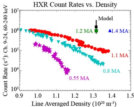
Fig.4.1 With increasing plasma current, the hard X-ray counts increase for high density. At 1.2 MA, the total HXR count is consistent with the model. The range of model values results from the uncertainties in the electric field distribution in the plasma.
