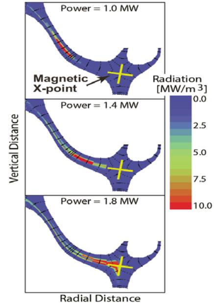
Fig. 5.3 Modeling of a double-null, long-leg X-point divertor for ADX-like parameters. Detachment is stable over a large range of parallel power into each divertor.
