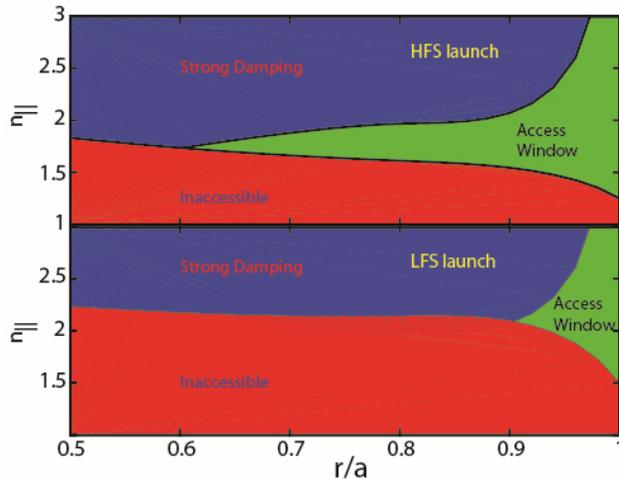
Fig. 4.2 Access window for HFS is dramatically improved compared to LFS LHCD launch using FDF profiles,  $B_0=6$  T and 5 GHz waves.
