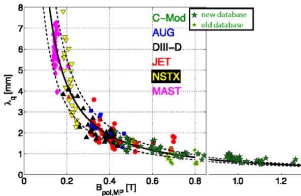
Fig. 5.1 Recent C-Mod data extends heat scrape-off width results to the ITER  $B_0$  (1.2 T) and beyond.
