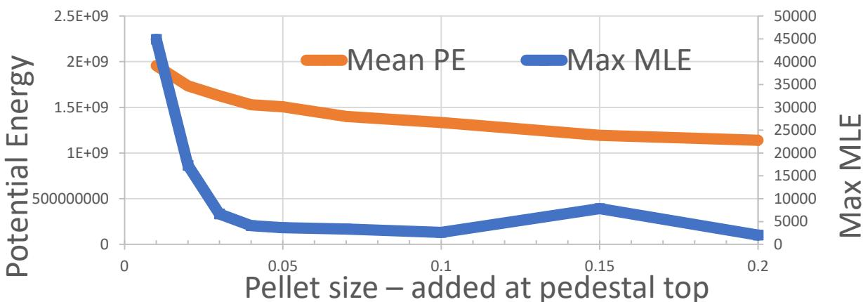
'Pelletizing' 2.5% pedestal fuelling to ITER relevant 45 pellets/sec, assuming ablation time of ~1ms, gives very similar results to constant fuelling ~ 99% reduction in avalanche size
