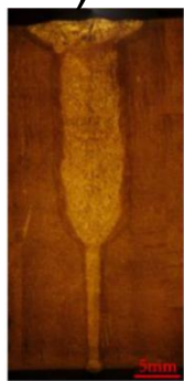
LB (30mm ) with filler wire
