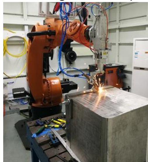
Submodule mockup welding
