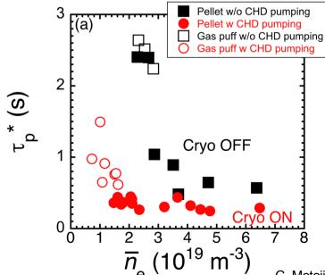
High performance of divertor cryo-sorption pump is realized in LHD.
