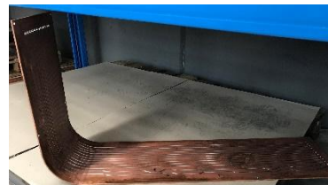
Plasma Box components and Faraday shield
