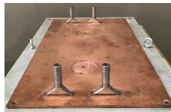
Plasma Box components and Faraday shield
