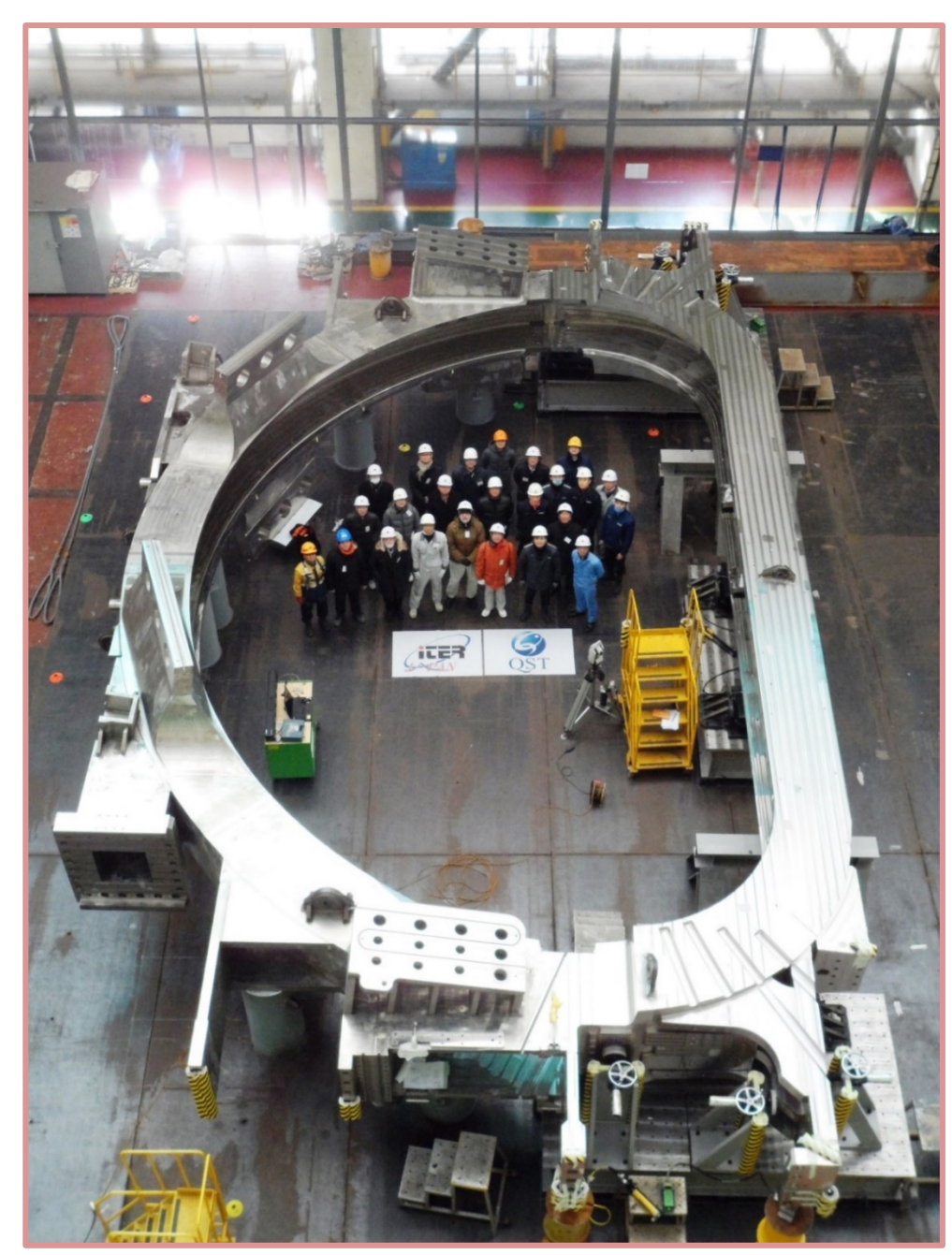
AU and BU after fitting up for the first EU products tested in horizontal position
