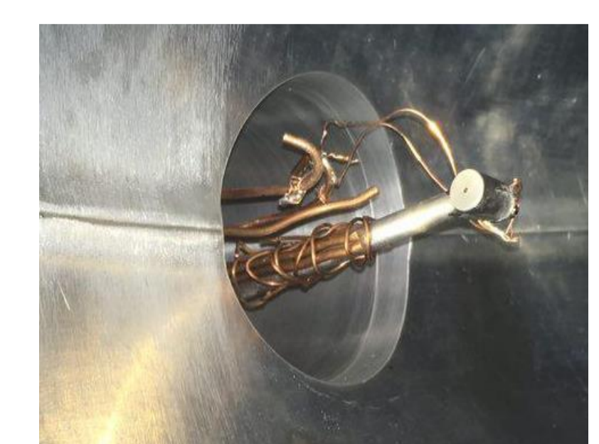
Figure 14. e-gun installed at SCR-1 stellarator vacuum vessel
