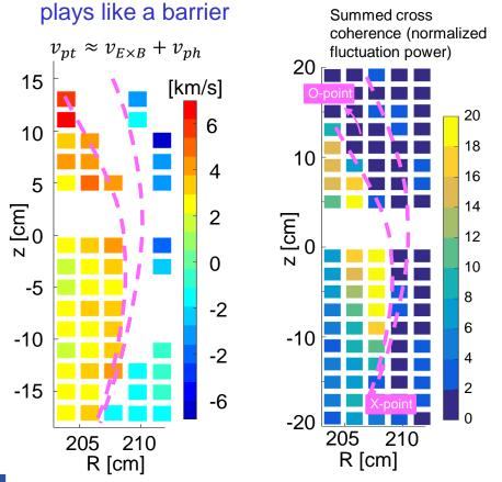
Minor disruption or the profile peaking can occur due to the strong turbulence outside the magnetic island
