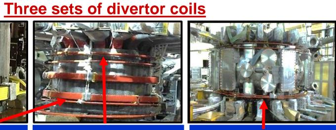
Main Divertor Coil (Inner) Aux. Divertor Coil (Inner)
