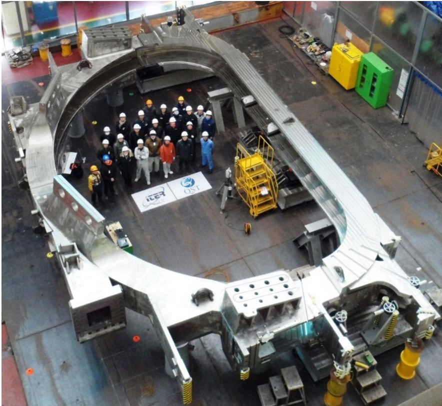
AU and BU after fitting up for the first EU products tested in horizontal position
