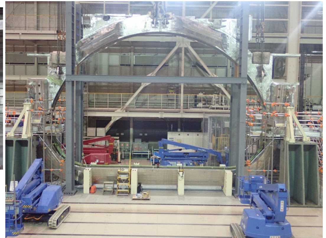
AU and BU after fitting up for the first JA coil tested in vertical position
