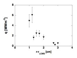
With an uncooled Liquid Li Limiter heat loads up to 5MW/m<sup>2</sup> were withstood for t=1.5s in FTU plasmas without any damage and low evaporation
