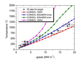
Experiments on PILOT-PSI have shown that an actively cooled tin limiter can operate at much lower temperatures than  $1000^{\circ}$  C for heat loads of 10 MW m<sup>-2</sup> as expected in FTU, sufficient to keep evaporation to below an acceptable level.
