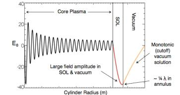
RF rectification, observed in divertor of NSTX, is converting wave power into spiral heat flux
