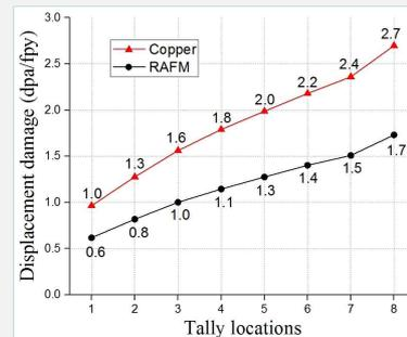
The copper material shows much lower displacement damage rates comparing with other parts since it is less exposed to the neutrons in the plasma.
