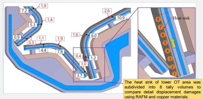
➢ The maximum damages are indicated in the RAFM heat sink material of upper OT area with a value of 10.9 dpa/fpy. Although RAFM was further away from the plasma, the displacement damage on RAFM (10.9 dpa/fpy) was higher than tungsten (2.6 dpa/fpy). This is due to the lower threshold energy of RAFM than tungsten (RAFM ~40 eV, W 90 eV).
