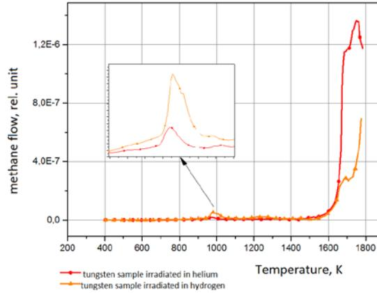
FIG. 7. Dependence of change in methane partial pressure from sample temperature in working chamber of experimental facility
