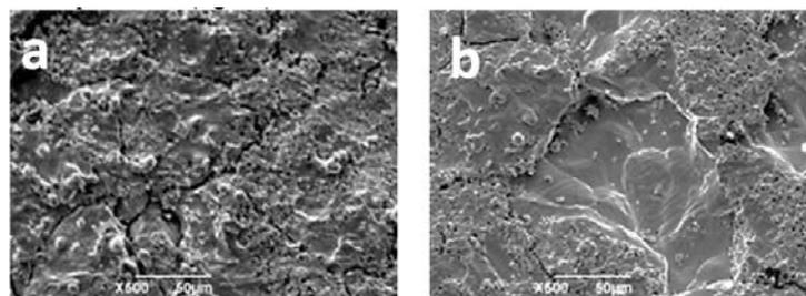
FIG. 5. Comparison of the surface microstructure of the tungsten samples with unpolished surfaces irradiated in hydrogen and helium: T5 DF (H) and R8 DF (He)
