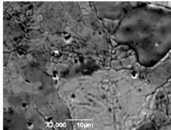
FIG. 2. The typical microstructure of the surface of the tungsten samples irradiated in hydrogen: sample U5 DF – pores of 1-3  $\mu\text{m}$ .
