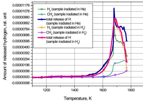
FIG 8. TDS dependencies of hydrogen gases release from tungsten samples.
