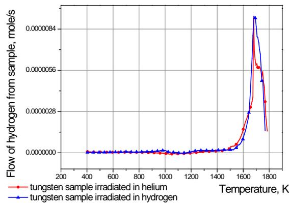
FIG. 6. Dependence of change in hydrogen partial pressure from sample temperature in working chamber of experimental facility
