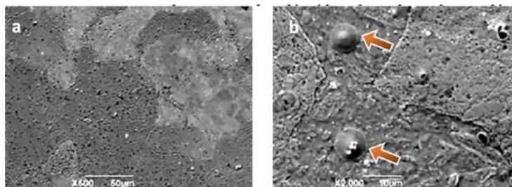
FIG. 3. The microstructure of the surface of the tungsten samples irradiated in hydrogen: formation of pores (a - S8 DF) and blisters (b- R5 DF)
