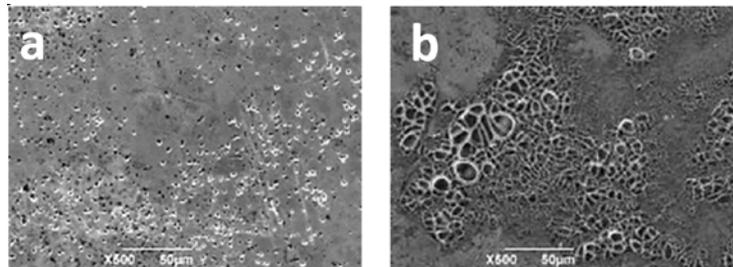
FIG. 4. Features of the surface microstructure of the tungsten samples irradiated in He: formation of micropores (a – S4 DF) and thin films (b – V6 DF).
