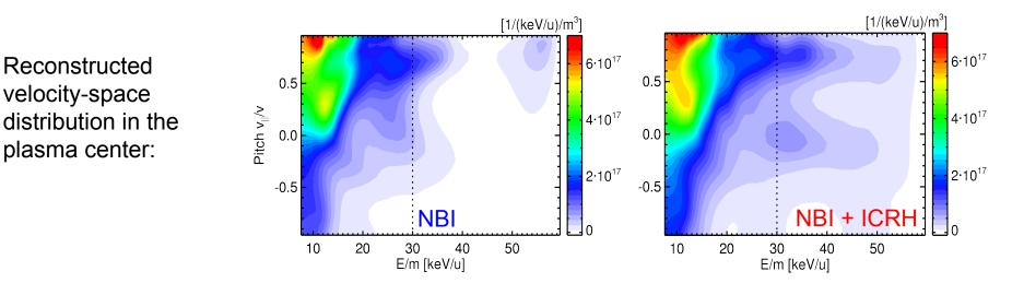
$\rightarrow$  Effect of ICRH is clearly seen: Significant high energy tails at pitches 0.7 and -0.1
