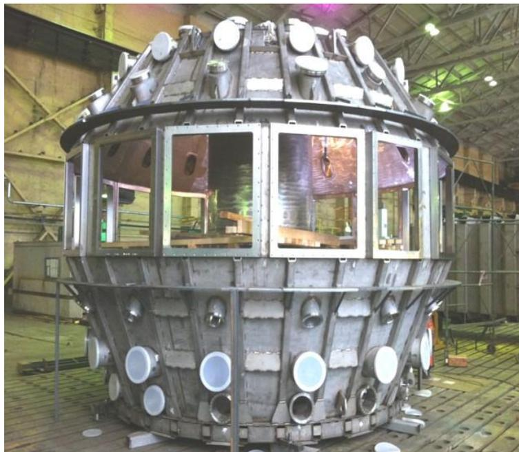
FIG.6. Vacuum vessel shell.
