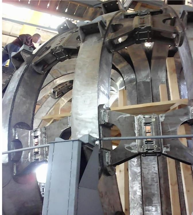
*FIG. 4. TF coil assembly with inter-coil mechanical structure.*
