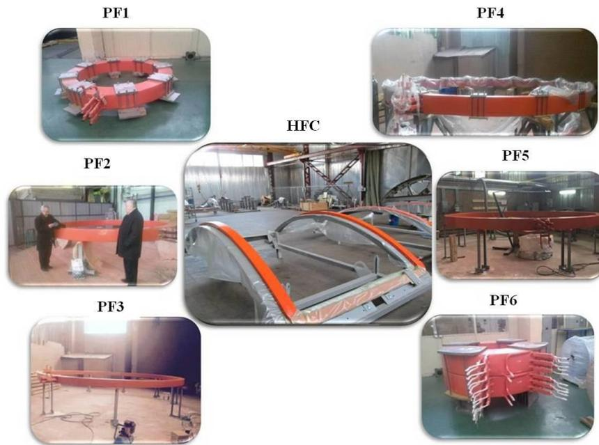
FIG.3. Poloidal field (PF1-6) coils and HF coils.
