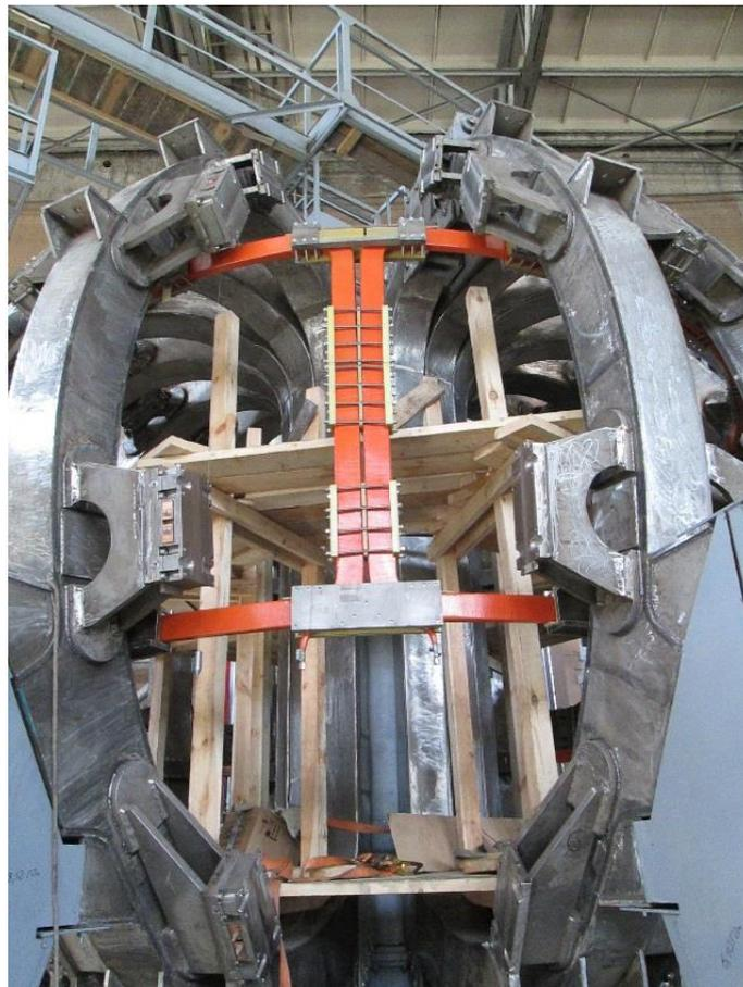
*FIG. 5. Placement of HF coils inside toroidal winding.*
