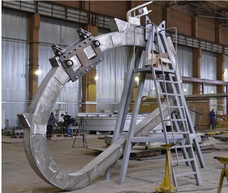
*FIG.1. Coil of toroidal field winding at plant in Bryansk.*
