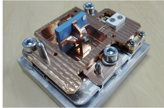
FIG. 19: Prototype in-vessel magnetic pickup coil support assembly (IO-CT, EU DA, Consorzio RFX).
