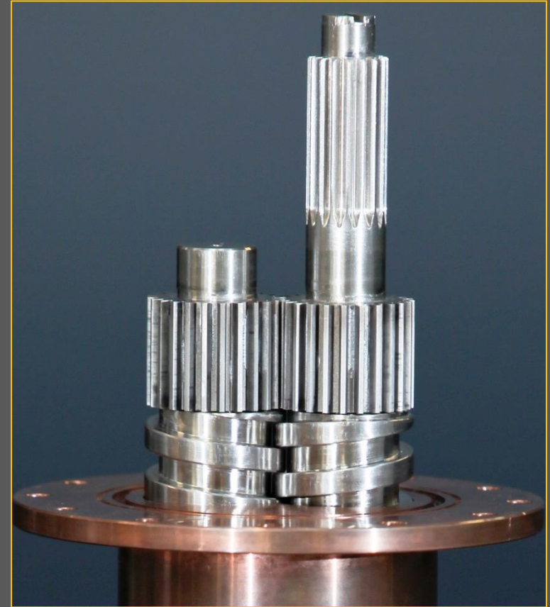
View of the drive shaft gears and top of the twin-screw extruder mechanism.
