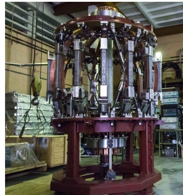
Globus-M2 toroidal magnetic field coil assembly together with central solenoid and supporting structure in the machine hall (Ioffe Institute, St. Petersburg, Russia).
