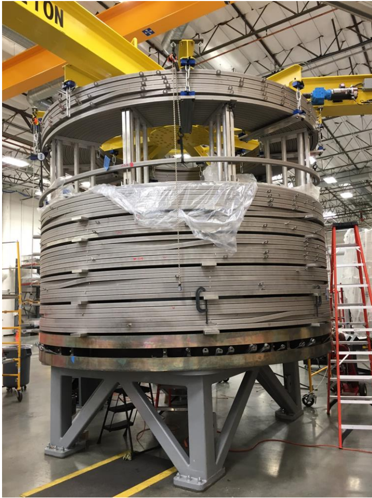
First production module in joining station
