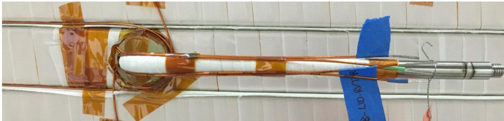
Quench detection wires exit along helium pipes
