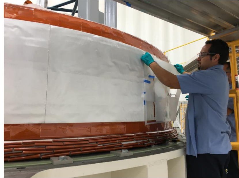
Sheets of ground insulation being applied to qualification coil
