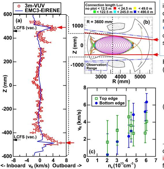
Vertical profiles of VUV lines from impurities emitted in the ergodic layer of LHD were measured by a spaceresolved VUV spectroscopy.
