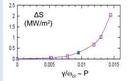
Calculated change of the energy flux across the Alfven resonance (resonant power absorption) vs  $\gamma$ .
