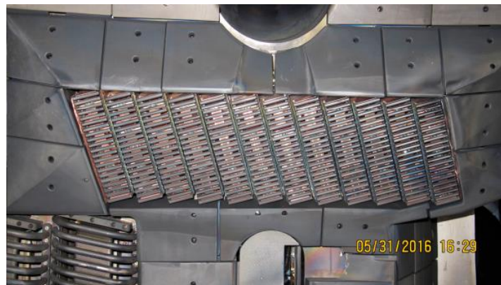
Traveling Wave Antenna in DIII-D
