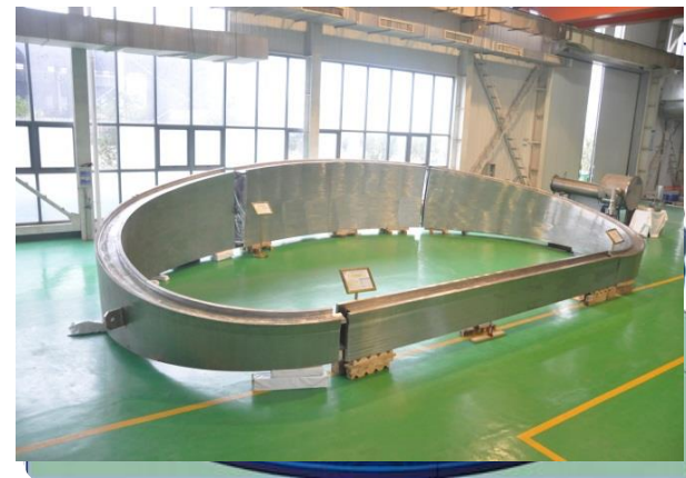
Assembly of VV Poloidal Sectors
