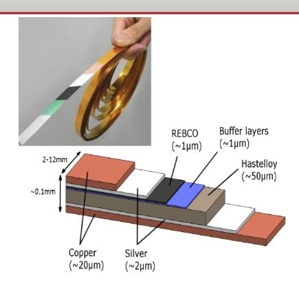
New REBCO high-temperature superconductors more than double the magnetic field previously available
