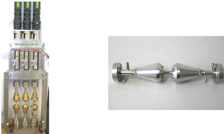
FIG. 3. Left:CFTM test frame. Right:Detail of specimen holder with tungsten heater bodies
