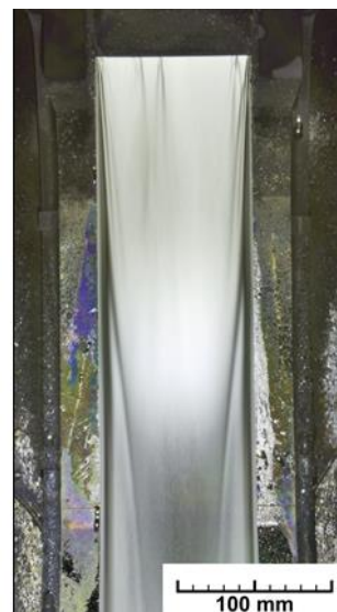
FIG. 1. Left: ELTL lithium loop in Oarai. Right: 2s exposure of the Li flow at 15 m/s.
