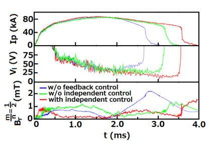
Time evolution of the plasma current, toroidal loop voltage and m/n=1/2 mode amplitude measured with sine and cosine coils for Br on the outer surface of the vessel. A slight increase in Br with previous feedback control (green), is suppressed in the current rise phase by modifying the control system (red), indicating successful compensation for the sideband effect.
