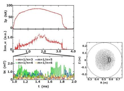
Time evolution of the dominant and secondary mode amplitudes in deep-reversal (F~-0.8) discharge, showing spontaneous growth and decay of the dominant mode. A Poincare plot of the magnetic field lines during the QSH at 1.7 ms in the right hand side trace shows recovery of the closed magnetic surfaces.
