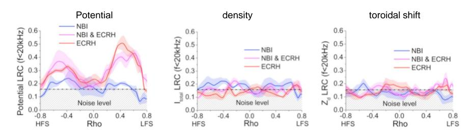
Experiments with combined NBI and ECR heating have shown evidence of the influence of ECRH on the level of broad-band plasma fluctuations and Long-Range-Correlations (LRC):
