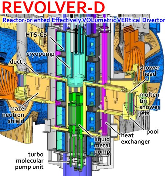
New ergodic limiter/divertor concept with showers of molten tin sheath jets is proposed for the LHD-type helical reactor FFHR-
