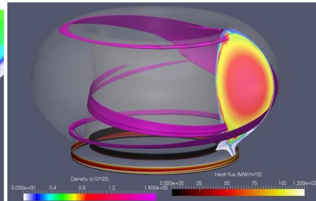
**Figure 4:** The pellet cloud distribution during the pellet triggered ELM is shown in a pink band. The profile of the heat flux on the outer divertor target by pellet injection of 4.7mm pellet is shown in the color scale on the divertor. The toroidal asymmetry of the power deposition by pellet injection is observed.
