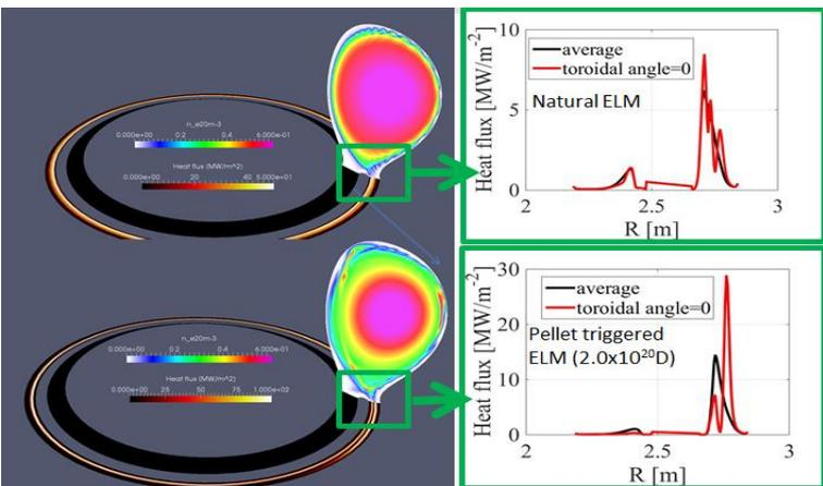
**Figure 2:** The heat flux on the divertor target during (top) the spontaneous ELM and (bottom) the pellet triggered ELM. The profile of the heat flux caused by the spontaneous ELM is toroidally symmetric.
