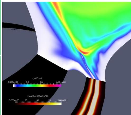
**Figure 3** The density contour and the heat flux on the divertor target. The density perturbation due to the pellet ablation creates a secondary connection of the particle/heat flux on the divertor target.
