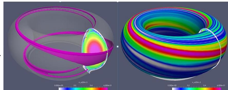
**Figure 1:** The pellet triggered ELM in JET plasma. (left) The pellet cloud is shown in the pink band. The pellet from outer midplane ablates and the pellet cloud expands along the magnetic field line. (right) The density contour plot on the separatrix. The filamentary structures caused by the pellet are observed.
