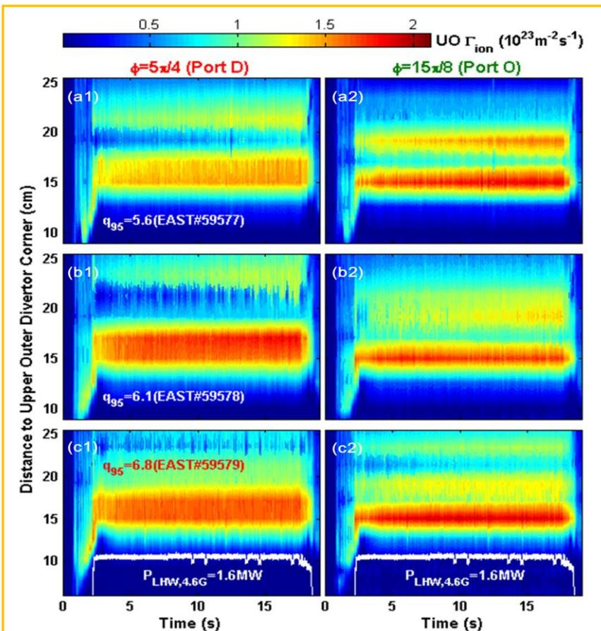
2D contour plots of measured particle fluxes on upper outer divertor target in Port D&O for three long-pulse discharges of different  $q_{95}$  in quasi-DN configuration.  $P_{LHW, 4.6GHz} \sim 1.6MW$ .
