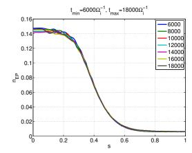
FIG. 11.: EP radial redistribution in time for a simulation where both the continuum mode (n=6) and the zonal structure (n=0) are kept.
