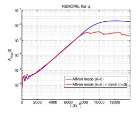
FIG. 8.: Vector potential measured at s=0.5,  $\chi=0$ , for the linear simulation, the nonlinear simulation with only the continuum mode with n=6, and the nonlinear simulation with both n=6 and n=0.
