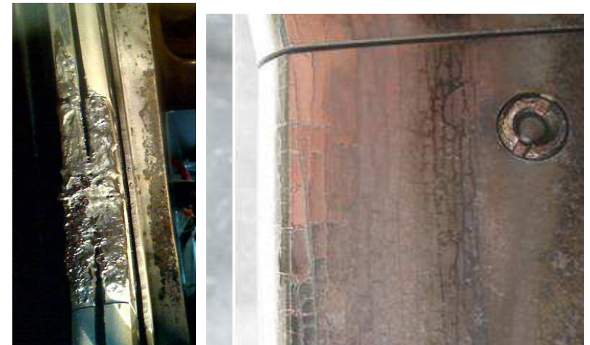
Effect of plasma exposition on limiter plates of ITER-grade tungsten studied.
