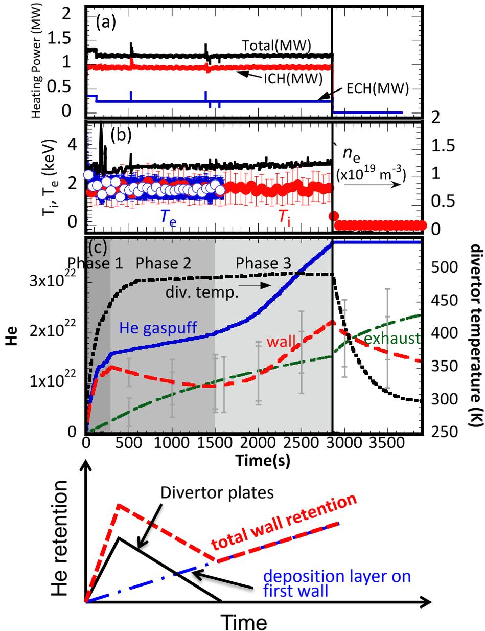
**Wall does not saturate during 48 min. discharge due to deposition layers**
