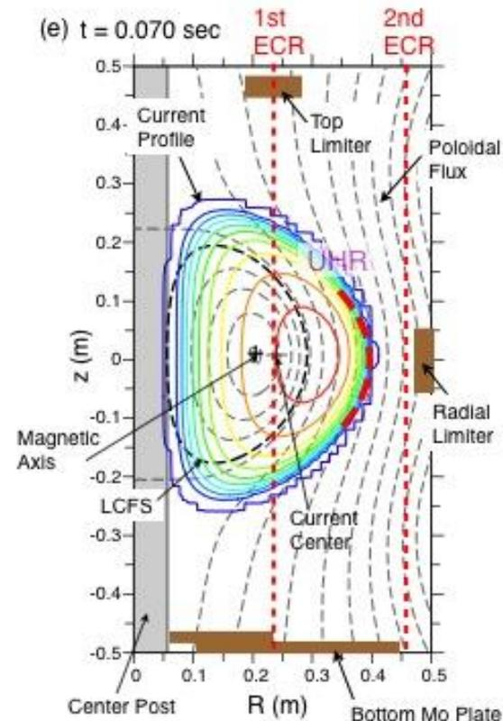
Density and soft X-ray emission increases when the  $2\omega_{ce}$  layer is located on the outboard side of the upper hybrid resonance (UHR) layer, i.e., when EBW is excited in the 1<sup>st</sup> propagation band. Such  $B_t$  dependence is observed at two different microwave frequencies.
