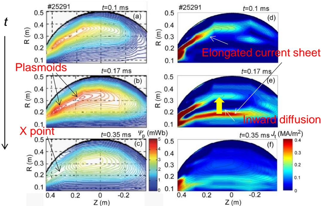
1. Formation of closed flux surfaces (c) was verified. The ratio of the closed flux to the total flux is 25-30%.
