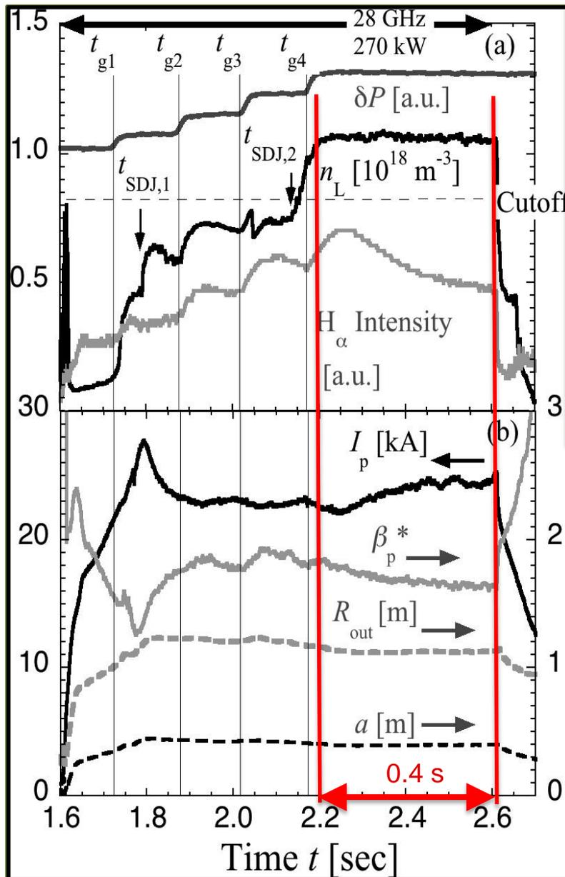
Microwave power was injected at two frequencies (8.2 GHz and 28 GHz) simultaneously for fully non-inductive  $I_p$  start-up and sustainment in QUEST.
