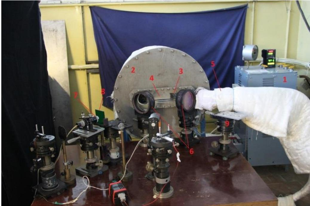
*Fig.3. Installation for FM mockups tests under water pressure and heating. (1) hydraulic and heating station; (2) vacuum vessel; (3) quartz window; (4) FM mockup; (5) water pipeline; (6) lenses; (7) test object; (8) "green" light filter; (9) camera holder.*
