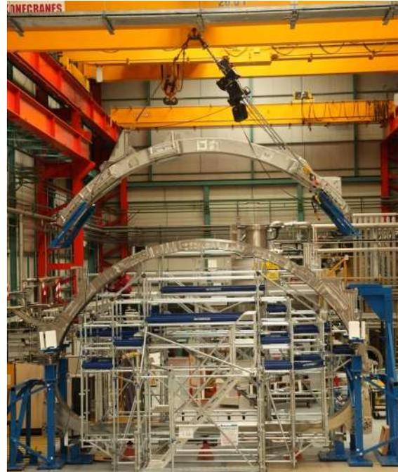
Fig.9: the 1st validated TF coil during assembly with its OIS at CEA/Saclay.
