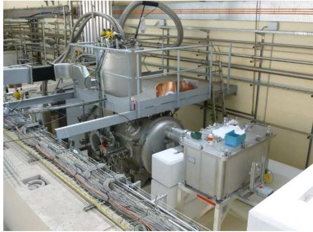
Fig.8: Sathori cryostat connected to cryogenic lines through Cryholab at CEA/Saclay.
