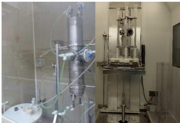
*Fig.7: pre-series cavity preparation: chemical etching (left) and high pressure rinsing (right).*
